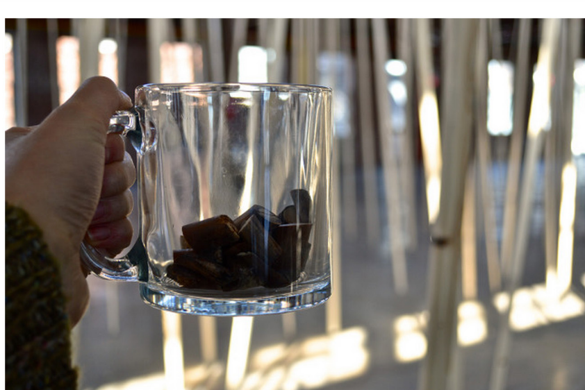
Knots that have popped out from the the wood beams over the course of the installation
